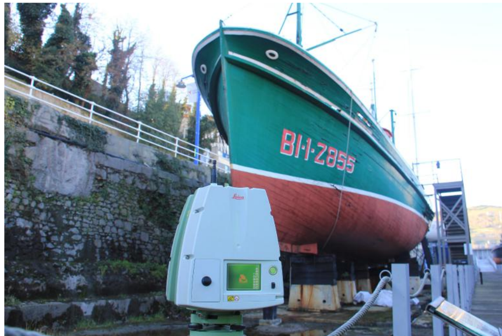
One of the stations for hull recording: the image created can be seen on the screen (J.M. Matés Luque)
