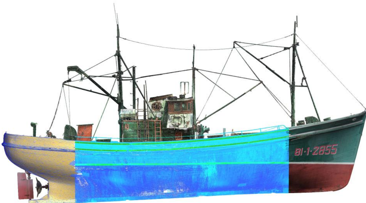
The 3D mesh, the colourless point cloud and the coloured 3D mesh combined (Oskar Moral Goirigolzarri)
