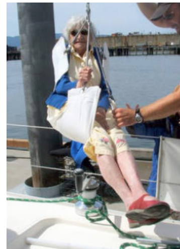
Bosuns chair or conventional sling using barge pulley system
