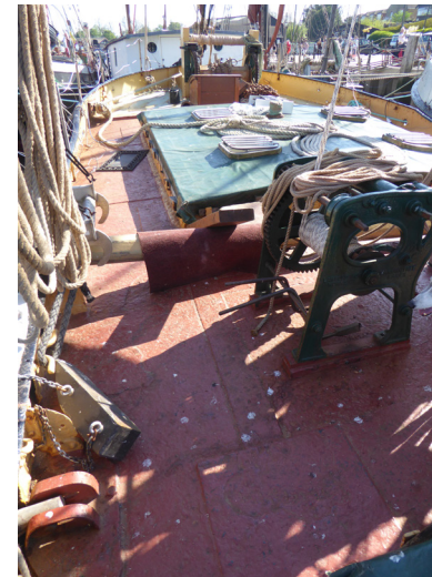
Comparable deck fit-out with ropes and self tacking (right image) headsail traveller
