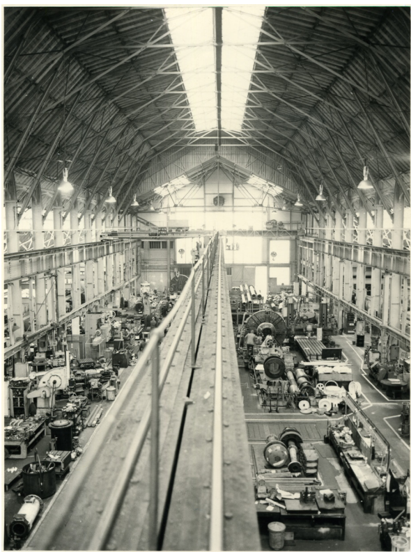
No 8 Machine Shop at Chatham Dockyard – a propeller shaft lathe dominates the top right hand corner of the workshop. PHA9486
