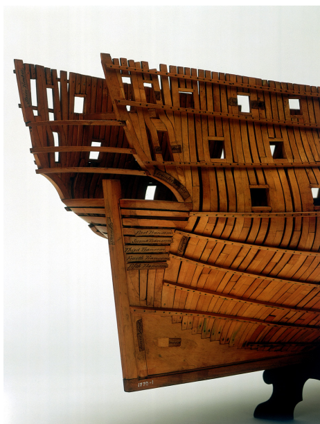
This model of a 74-gun ship, the Intrepid, was made to show to King George III c 1770, and the names of the individual timbers are marked on it.
