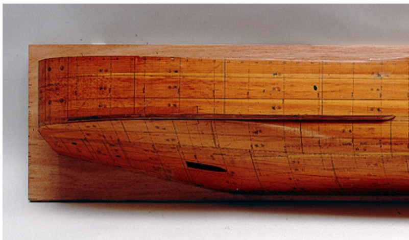
A plating model of the Bardic Ferry of 1957, the first purpose built roll-on roll-off or 'ro-ro' ferry.
