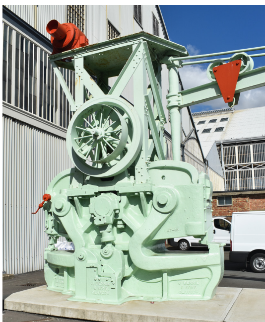
Punch & Shears – the punch is on the left hand side – the shears on the right
