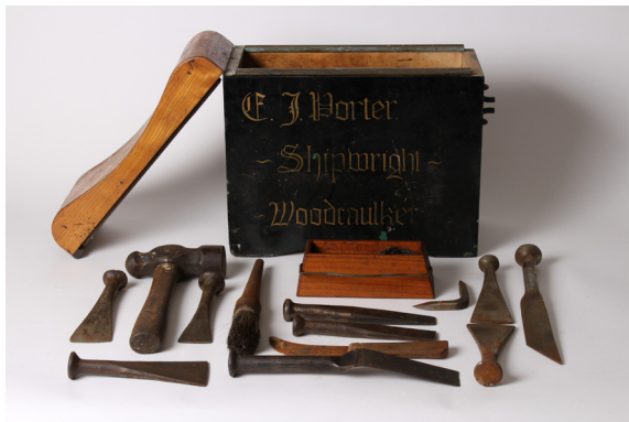
Caulker's box and caulking irons HTL497
