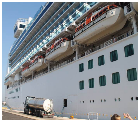
Modern ships' boats are usually lifeboats, though in the case of a cruise ship they can also be used to take passengers on trips, when they are known as tenders.
