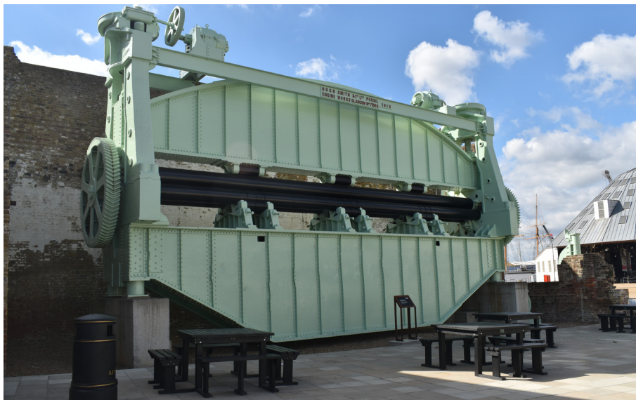
These 42ft plate bending rolls (made by Hugh Smith & Co, Possil Engine Works, Glasgow in 1913) were used to bend armour plate and steel for submarine hulls at Chatham Dockyard until its closure in 1984. This equipment weighs c 200 tons!
