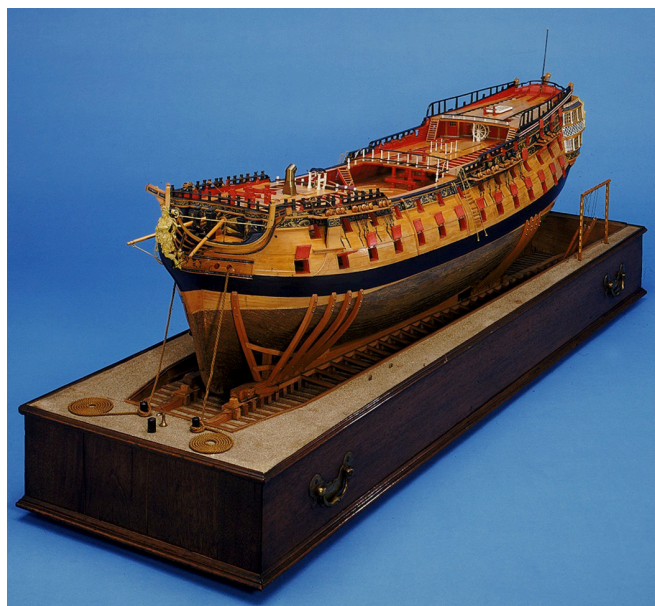
One of the best Georgian models is that of the Bellona, now known to have been made by Thomas Burkett, William Thompson of Chatham Dockyard in 1759–60. It is shown on its launching ways. Later the model was coppered and may have been taken to King George III to demonstrate the principle of coppering.
