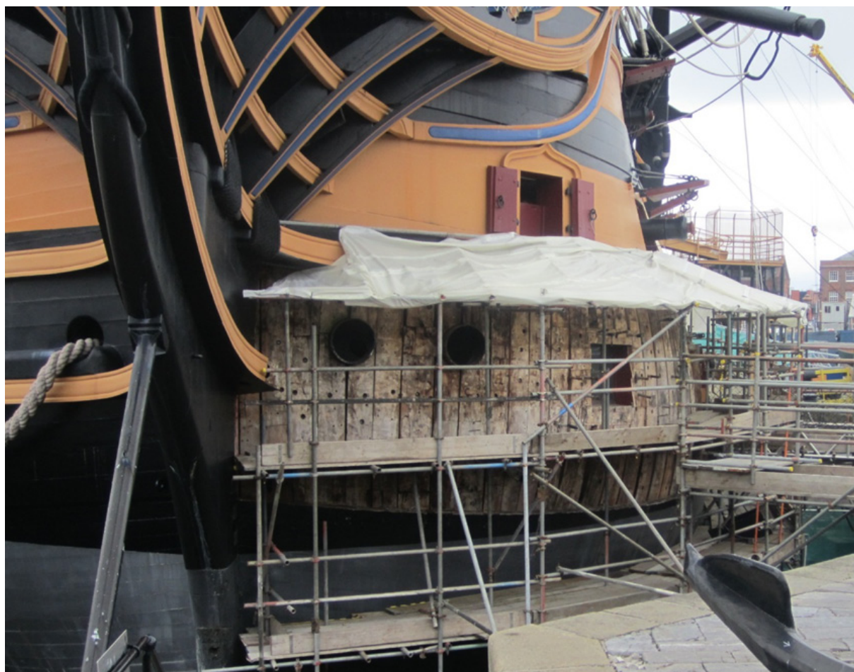
HMS Victory in 2012, showing the major restoration/reconstruction of timbers in the bow.
