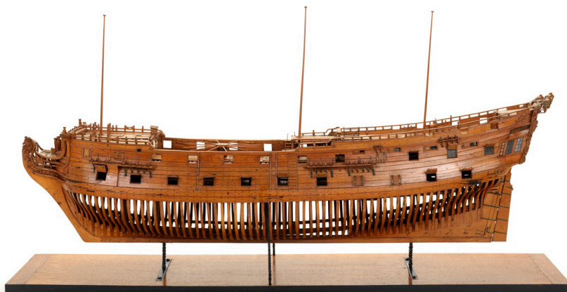
The classic style of Navy Board model, with open frames and planking above the wales. Warship, Fourth-rate, 50 guns c 1725 SLRo431 © National Maritime Museum, Greenwich, London
